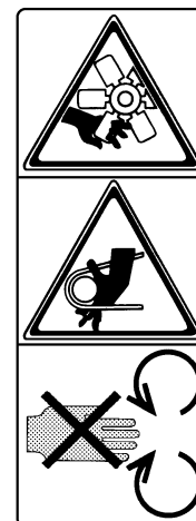
(4) Part No. 6C090-4958-2 Stay clear of engine fan and fan belt.
