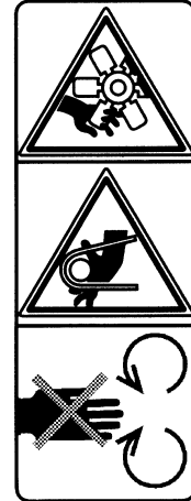
(3) Part No. K3111-6586-1 Stay clear of engine fan and fan belt.
