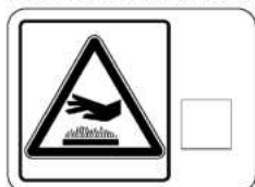
(3) Part No. 6F172-4719-3 Do not touch hot surface like muffler and so on.
