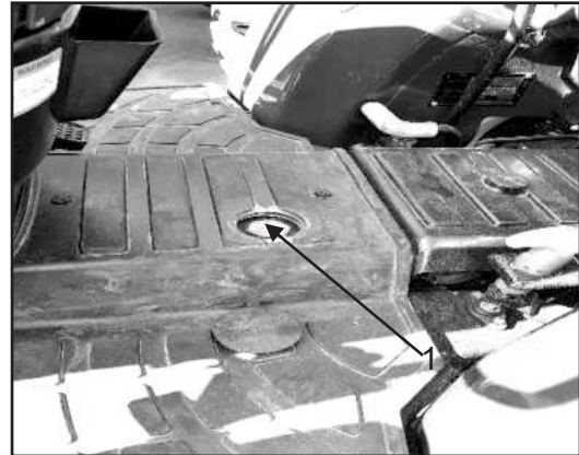
1. Transmission Oil Dipstick Cum Oil Filling Port
