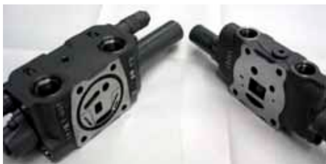
23.Inlet section (Travel independent valve) and travel R section.
