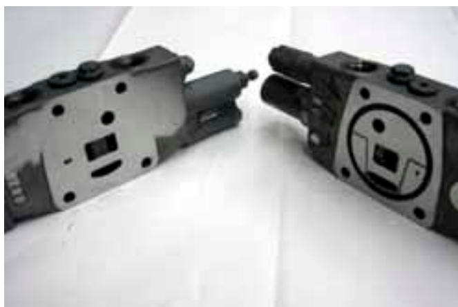
27. SP2 section and dozer section.
