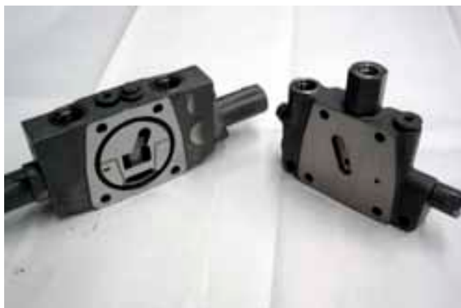
29. Swivel section and P3 confluence section.
