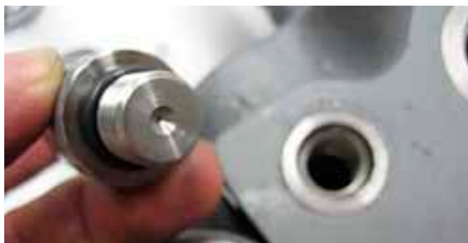
17. Plug with orifice ( P_{Ls} )
