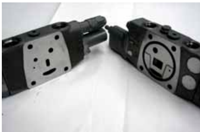
26. P 3 inlet section and SP2 section.
