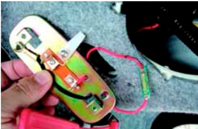
5. Wire harness for room lamp
