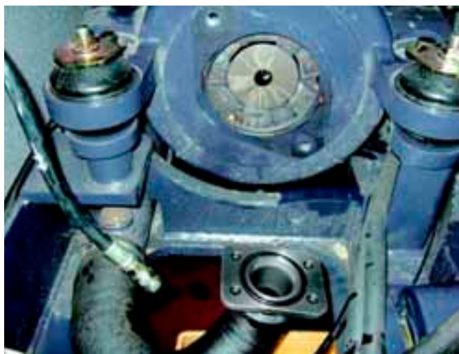
6. View after pump discounting.
