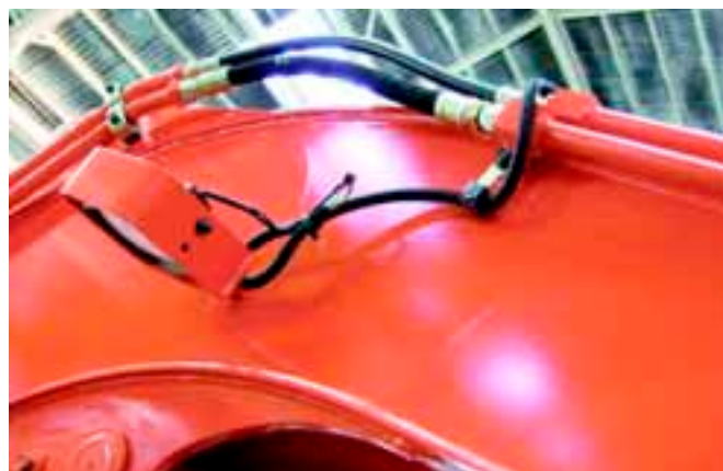
Work lamp harness
