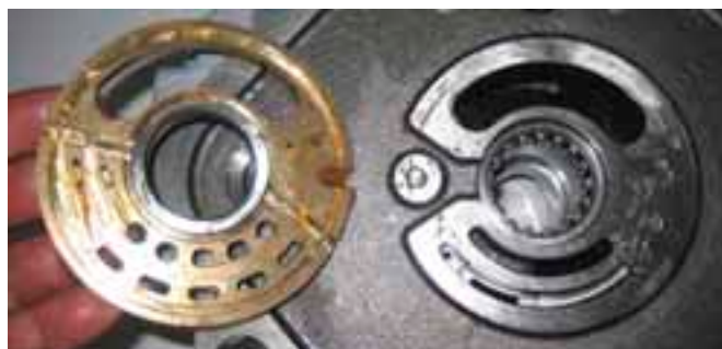
7) Take out the valve plate.
