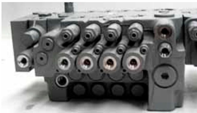
10. Side view, mono block pilot port.
