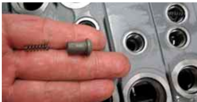
19. Load check poppet and spring.
