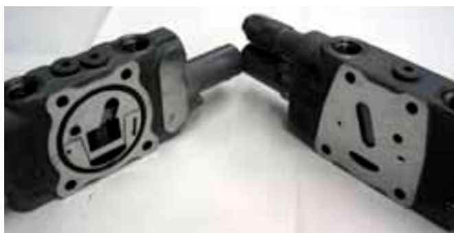
25.Travel L and P 3 inlet section.
